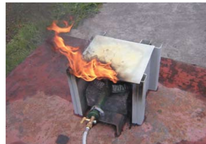
Normal Ampelite flat panel, 20 seconds after ignition.
