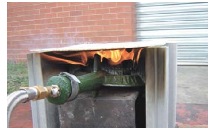
Ampelite fibreglass panel with the addition of the Fireshield tissue, 15 minutes after ignition. Note the lack of sooty black smoke (very impressive).
